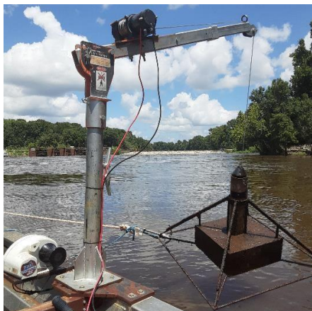
A mooring designed to hold one of the 24 Innovasea high residence receivers (HR3) deployed during the fine-scale acoustic study. The mooring was hand grappled, lifted with the capstan winch, and then connected to the rotational davit arm in order to maneuver the 300 pound mooring. Photo credit: Aaron Bunch
